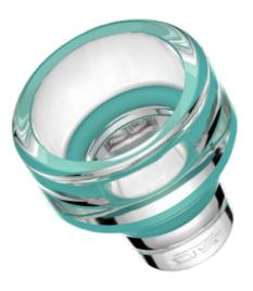
It is made of EVA (Ethylene Vinyl Acetate Copolymer) manufactured by DOW. It is not silicone resin and it is PVC, phthalates and bisphenol A free. It complies with European regulations for materials intended to come into contact with food and beverages. It is not glued to the closure, you can remove it by hand and recycle in the same way as low density polyethylene (used in juice and milk cartons).
